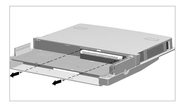
Figure 7-13. Removing the ISA Connector Board
